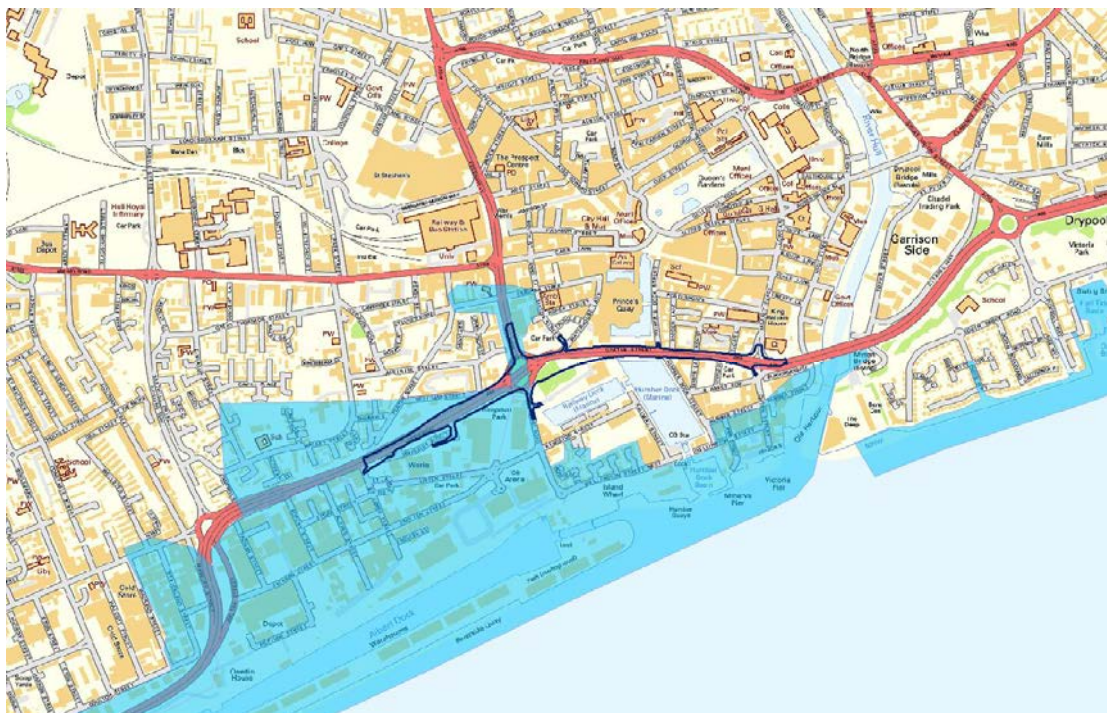
Figure 8-3 - Extent of flooding (blue shading) near the Scheme during the tidal surge of December 2013.
