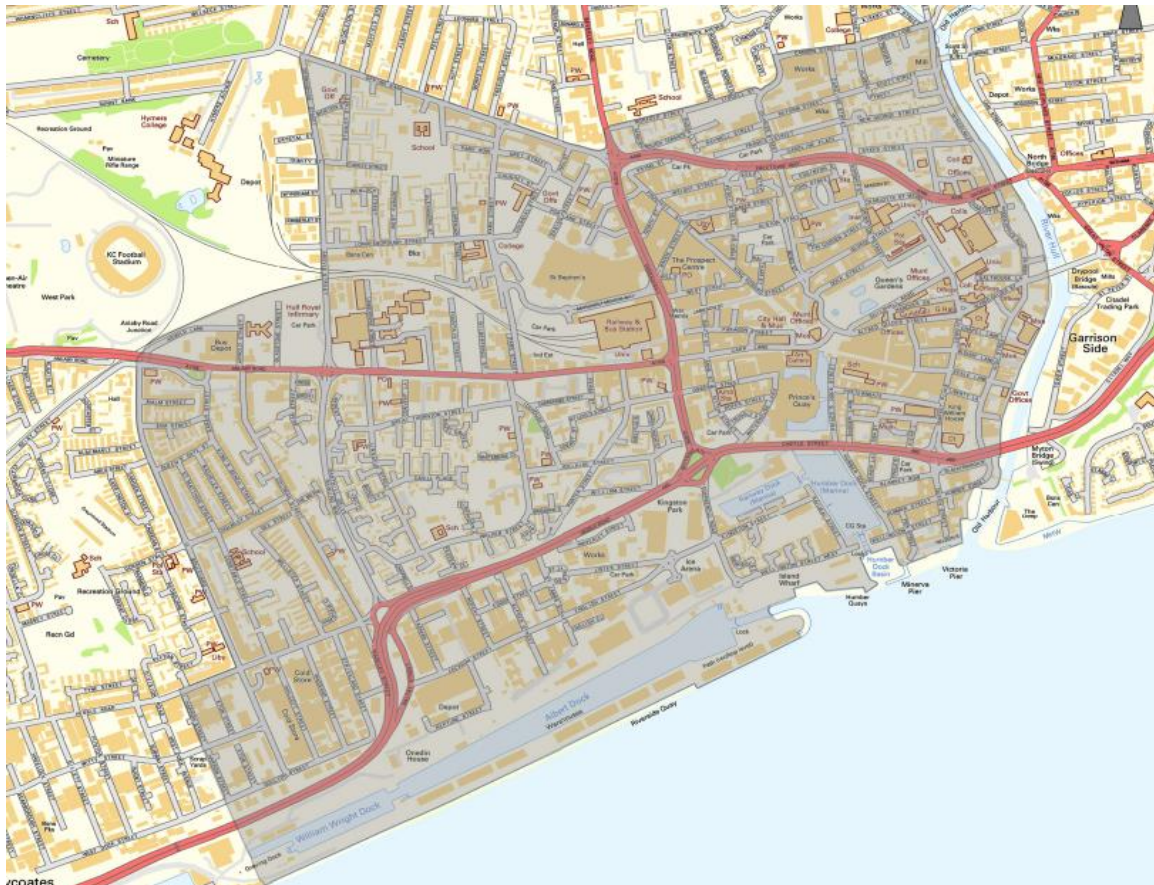
Figure 9-1 - Extent of the Flood Risk Assessment study area (2D zone in Infoworks ICM model).
