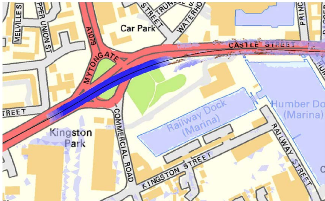
Figure 10-2 – Flow propagation for a 1 in 200-year Humber wave overtopping event at simulation time 15hrs 00mins
