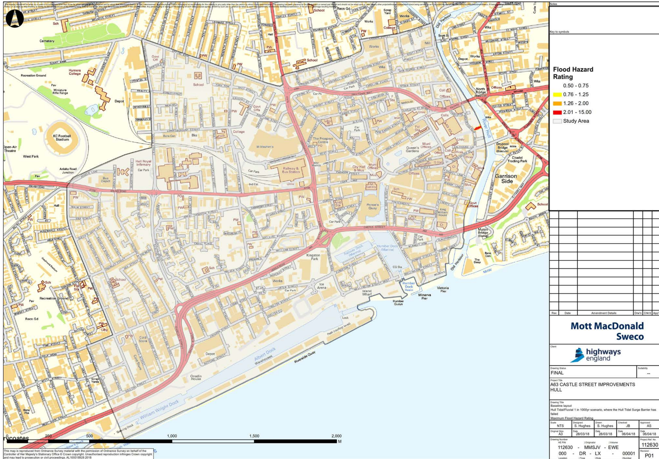
Figure 13.59 1 in 1,000-year River Hull tidal / fluvial flooding maximum flood hazard rating for existing layout (Hull Tidal Surge Barrier open)
